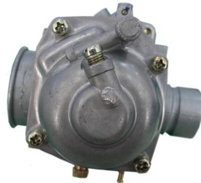
Remove the float setting bolt.
