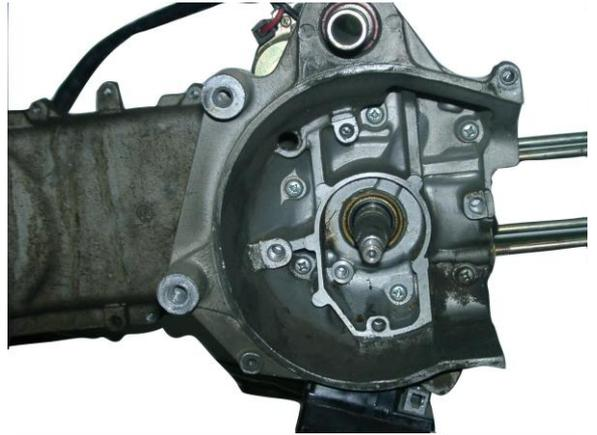
Remove the right crankcase from the left crankcase by using a pulley.
