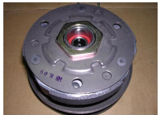
Fix the driven pulley in a compressor.
