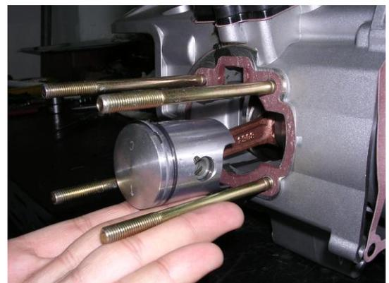
Install the cylinder gasket.
