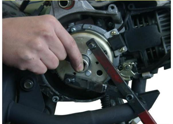
Remove the fly wheel by using a pulley.
