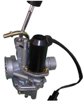
Remove the throttle valve from the throttle cable.
